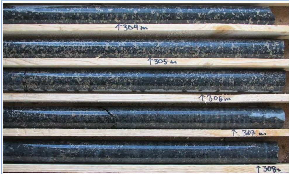
Figure 10: Mineralisation in diamond drill hole 13DDST009 303.5m – 308m 0.49% Ni and 0.42% Cu
