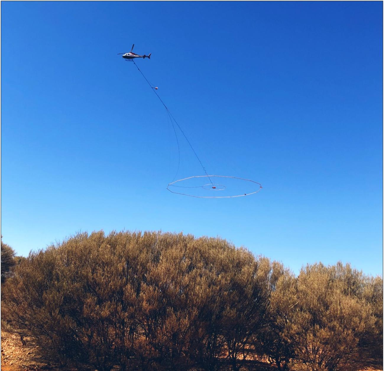
*Figure 2: Helicopter-borne VTEM™ survey in action over the Laverton Downs Project.*
