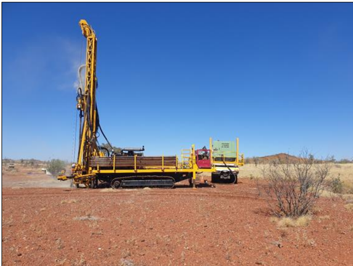
Figure 5: Track-mounted Combination RC - Diamond Drill Rig from Topdrive Drillers to arrive in early April
