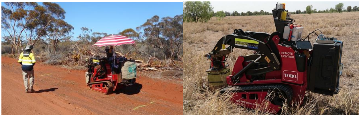
Figure 1: R&D Seismic Survey conducted by Ultramag enabled very low environmental impact seismic surveying at Carr Boyd, allowing the company to image the prospective basal contact at depth ahead of drill planning. The e-Vibe system enabled access into areas where traditional seismic systems were too large and destructive to operate effectively.
