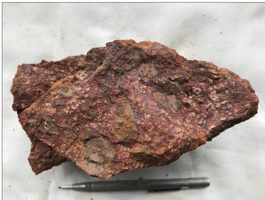
Figure 6: An example of strongly iron enriched, brecciated sedimentary rock from Frewena Frontier (South) with hematite-goethite cement and rimmed goethite clasts; sample location is shown by the white and red star in Figures 2 and 5.
