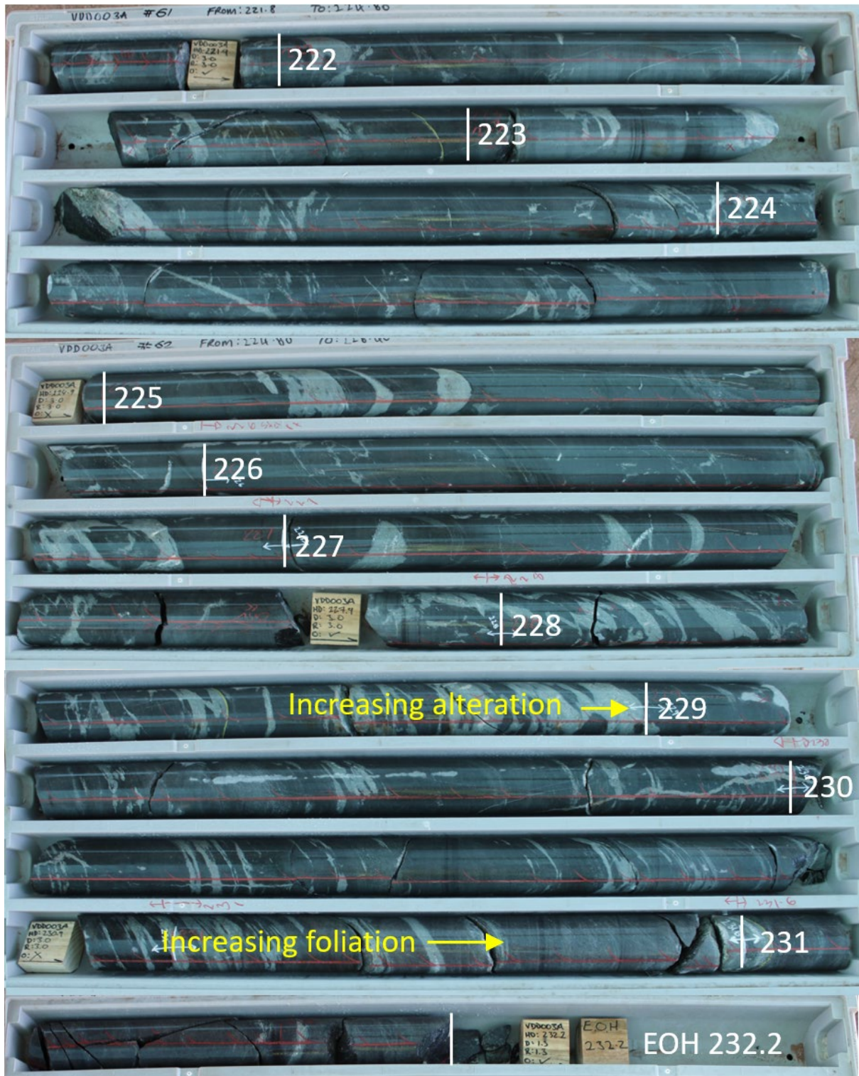
Figure 9; Core photos of alteration and hanging wall rocks intersected in hole VDD003A prior to intersecting the mine workings.
