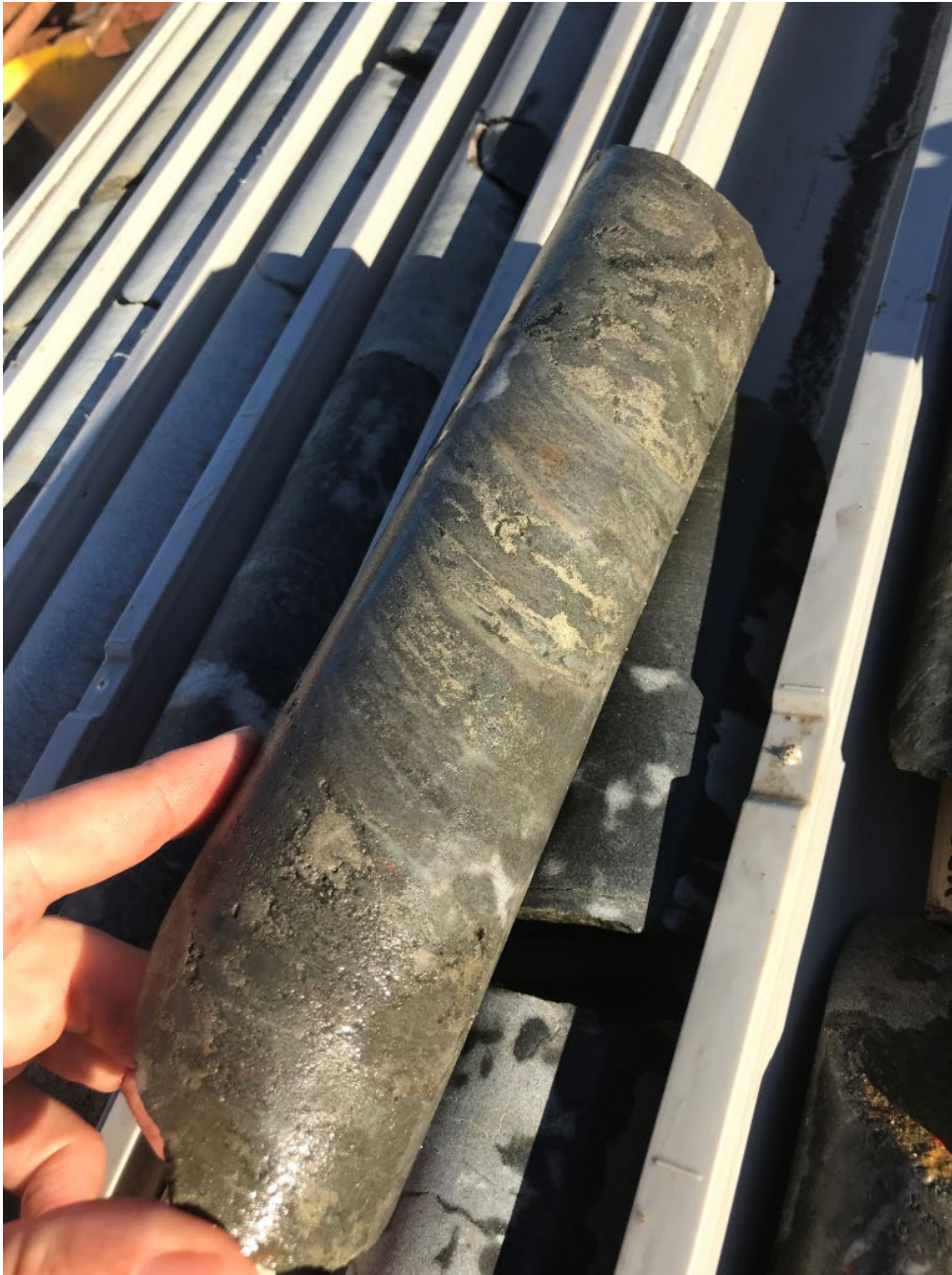
Figure 16; Sulphide rich (pyrite) shear zone encountered in hole VDD007 from 33.5 m.
