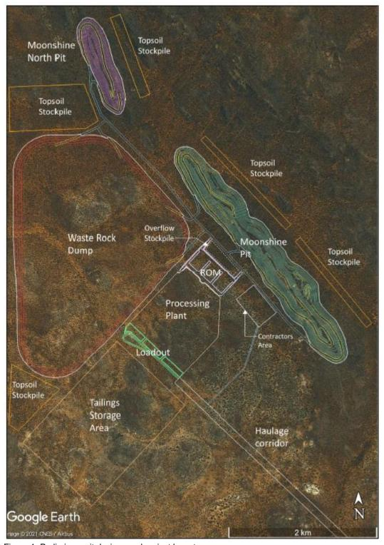
Figure 1. Preliminary pit designs and project layout.
