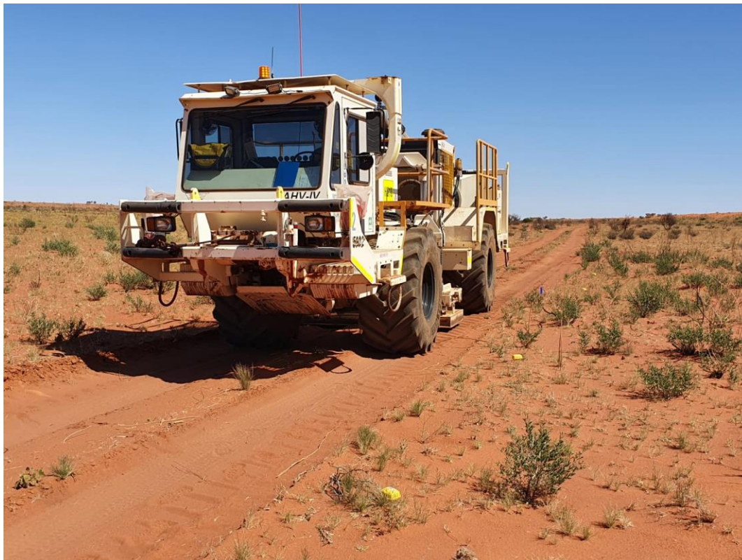
Figure 6 Hiseis Inova AHV-1V 62,000lb seismic vibrator truck with Inova Quantum receiver nodes layed every 5m along the track
