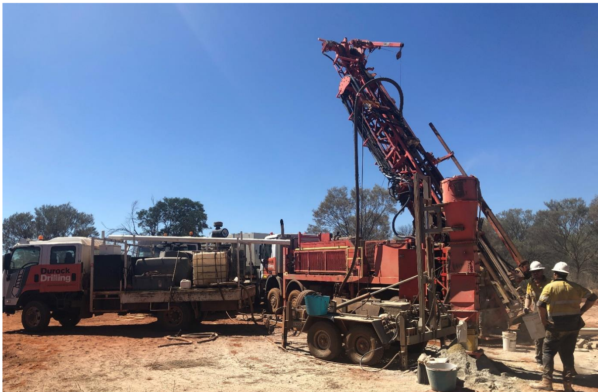
Figure 1 - RC Drilling underway at Reynolds Range April 2021
