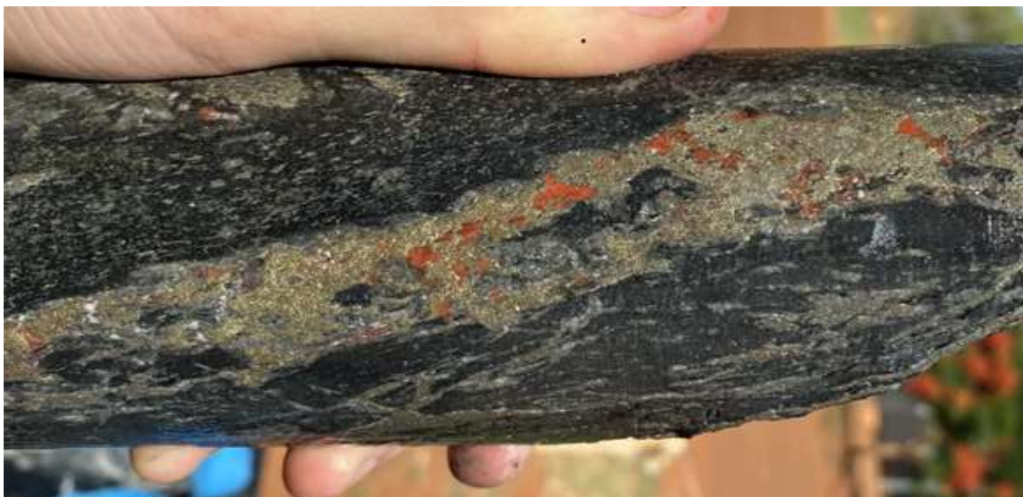
Figure 2: Example of a copper mineralised core from NDIBK04, depth 251m.
