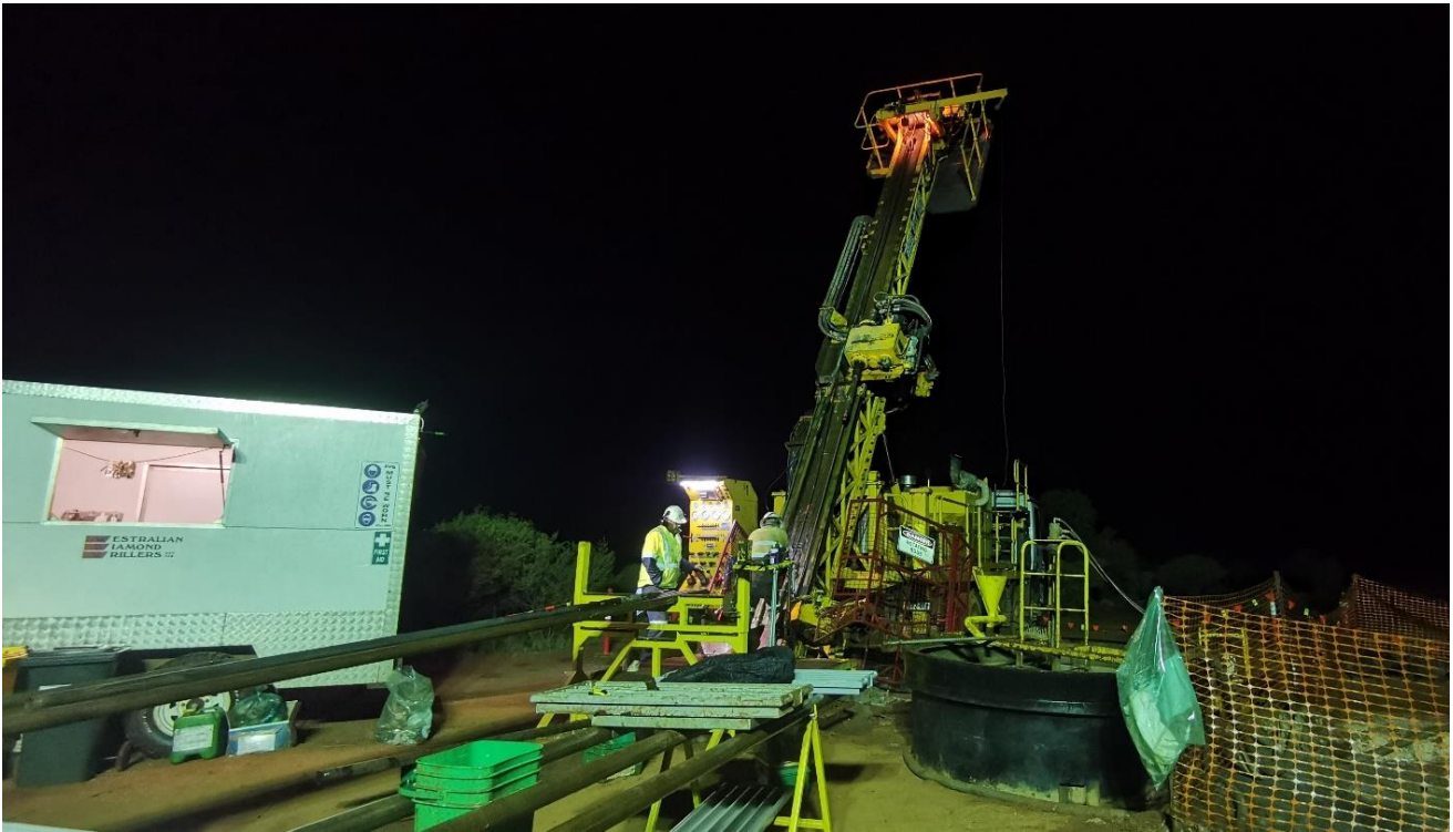
Image 4 - Nightshift diamond drilling at Mandilla East
