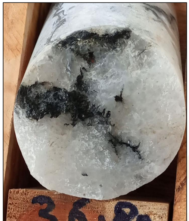
Figure 4 – Detail from CKDD002 at 37m showing tourmaline-pyrite mineralisation within quartz vein zone
