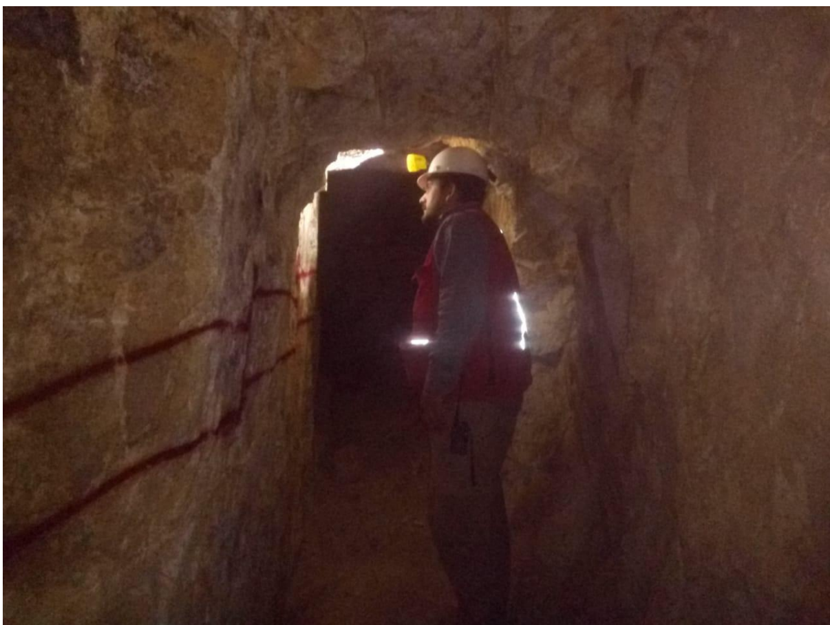
Photo 1 - Showing Channel marked in Magnata Access Drive wall prior to cutting with the Rock Saw
