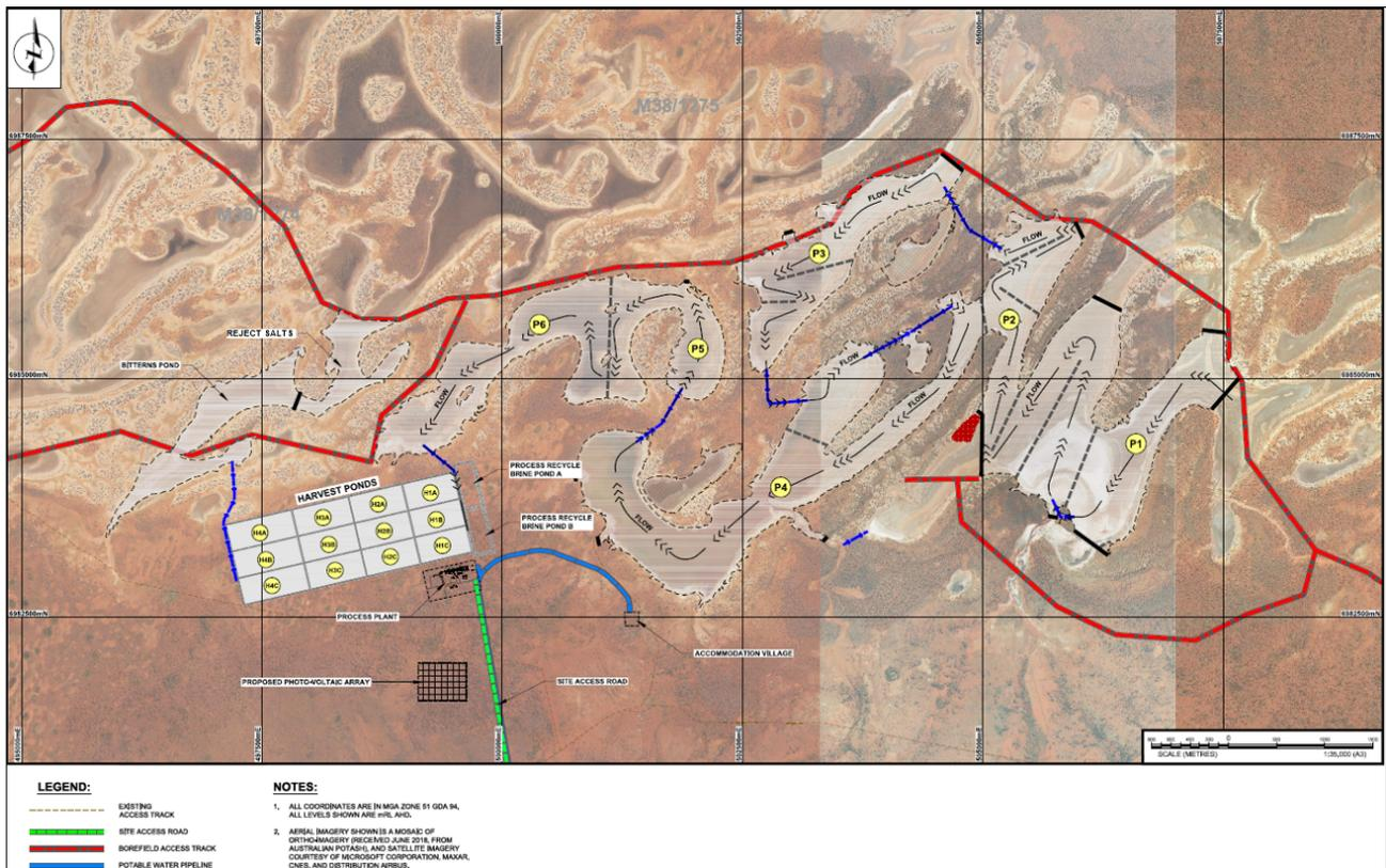
**Figure 29 Layout of pre-concentration, harvest and bitterns ponds**
