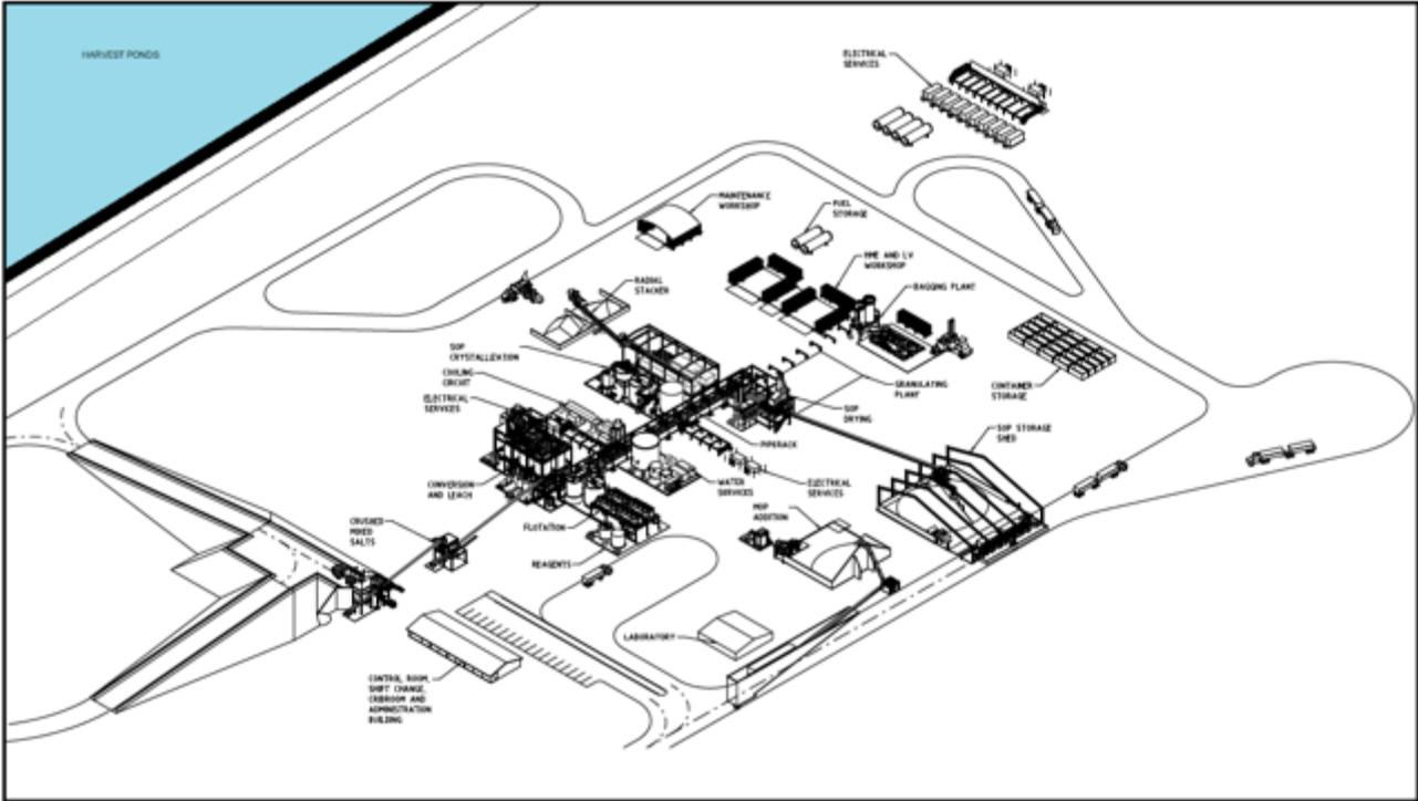
Figure 7 Schematic layout of LSOP process plant
