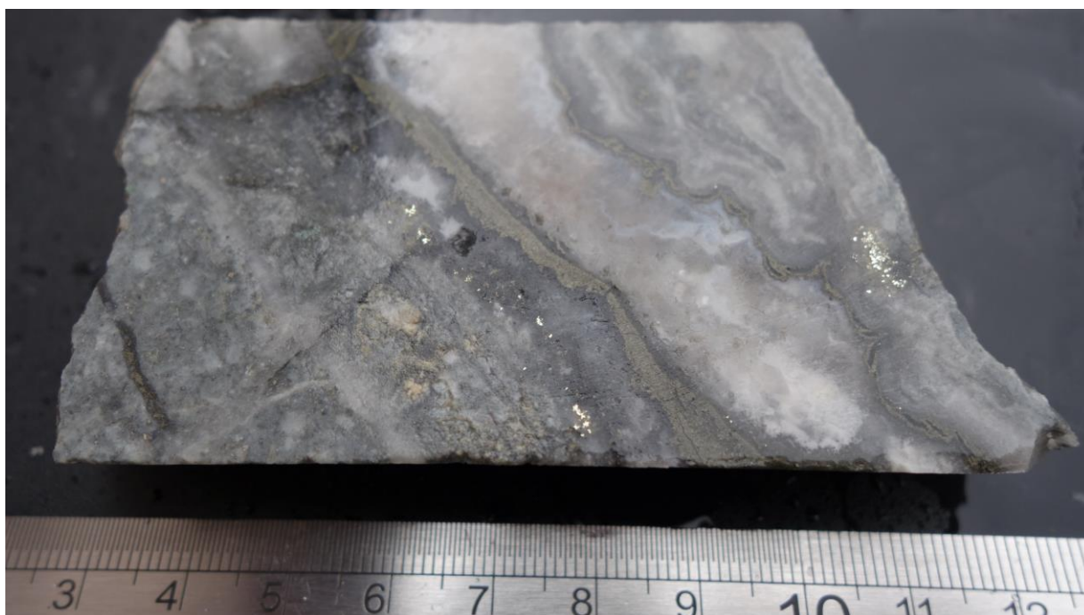
Figure 2: Visible gold in a ~5cm wide, drusy, fine grained, white to grey chalcedonic quartz-pyrite filled vein/stockwork zone at 41.4m in UGA-16, also visible on the surface cut core sample.
