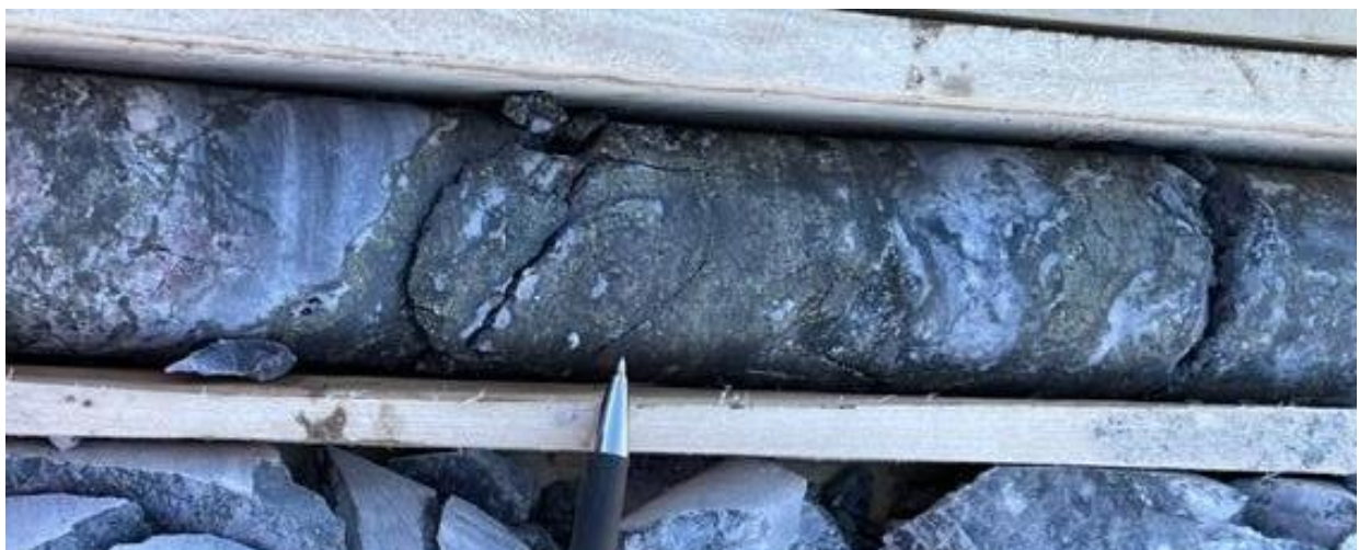
Photo 2 - GNDD-264 Limestone hosted skarn mineralisation 122 metres downhole
