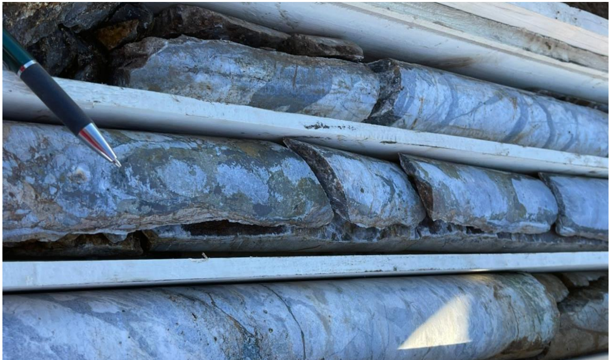
Photo 3 – GNDD-266 Limestone hosted oxidised skarn mineralisation; 38 metres downhole
