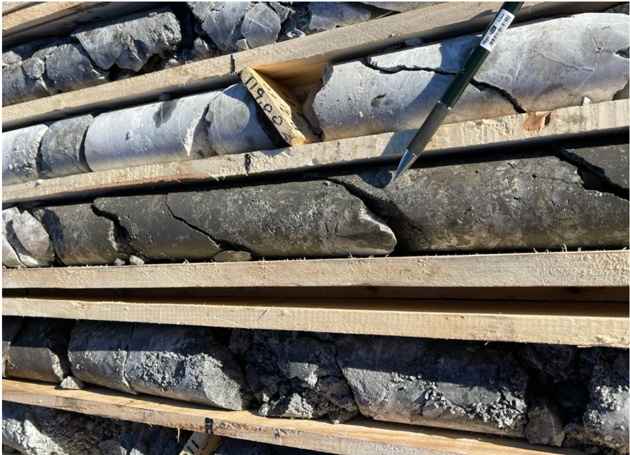
Photo 1 - GNDD-264 Limestone hosted massive sulphide skarn mineralisation 119 metres downhole
