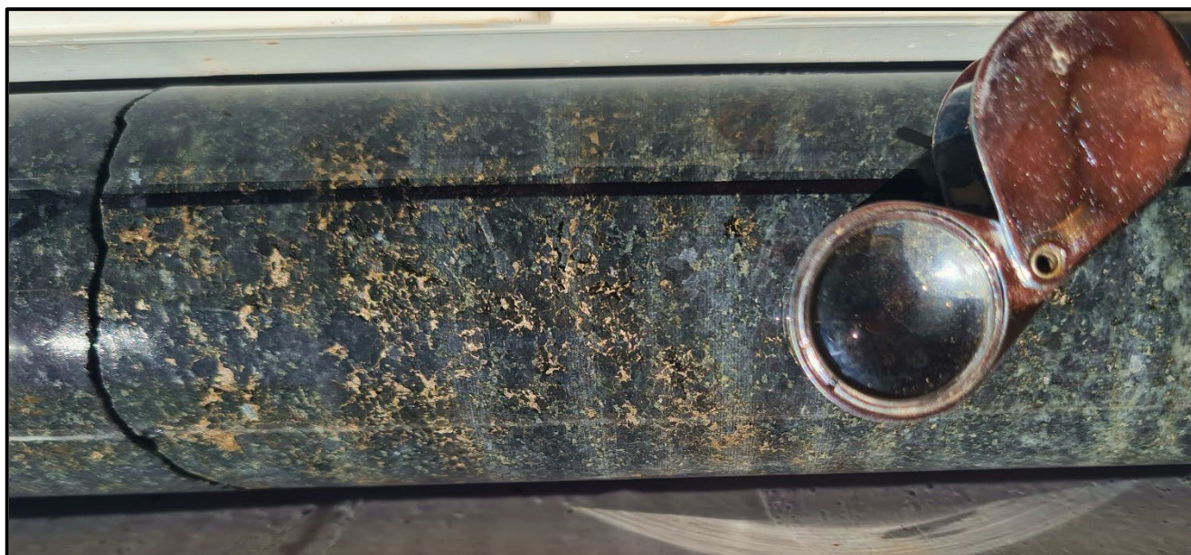
Figure 3 — Disseminated Sulphide in LADD003 at 170m (pyrrhotite with minor pentlandite/chalcopyrite)
