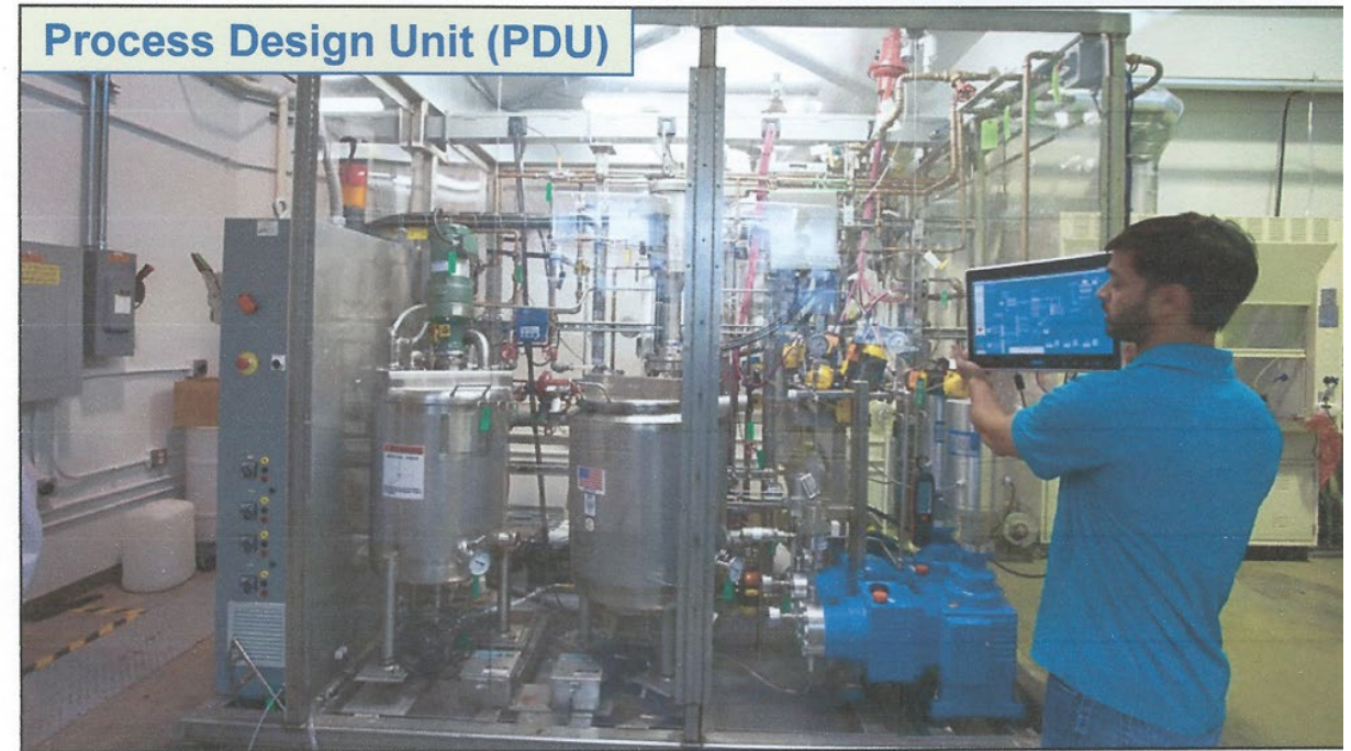
Scaled up OHD flow reactor designed by Australian scientist Ken Anderson, currently operating in Illinois State University USA
