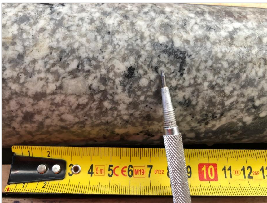
Figure 4. Endogranite with clusters of millimetric crystals of disseminated wolframite and minor cassiterite (21DD0008, 68.40m). This sample returned 0.22% WO 3 and 558ppm Sn over 3.00m.
