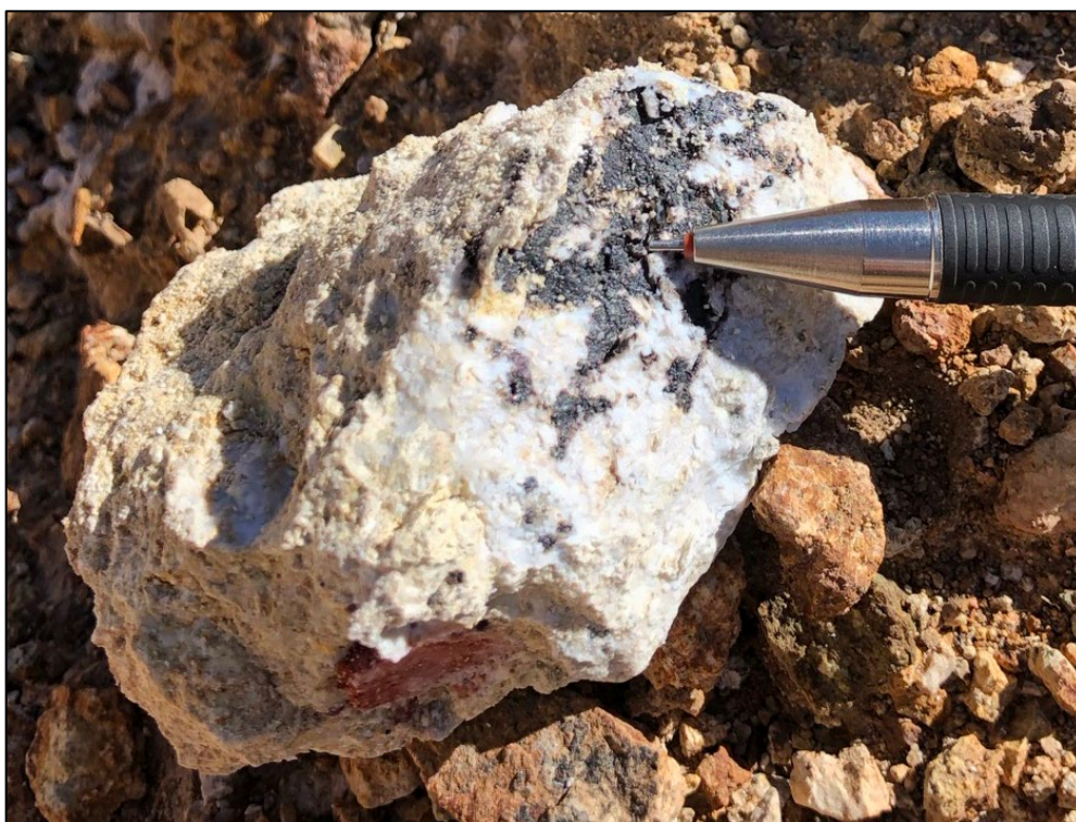
Figure 7. Hand specimen from the Loreto alteration zone showing intense argillic alteration (clay – silica – sercite) and neotocite (black copper oxide).
