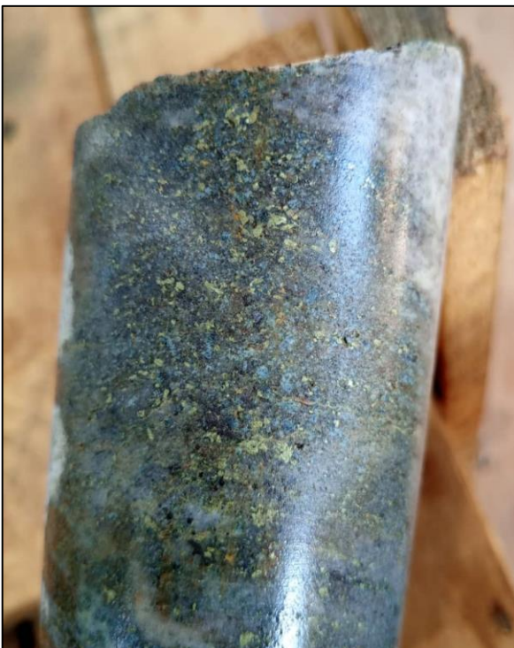
Figure 3 – Detail from CKDD003 (36m) exhibiting silicified metagranodiorite with up to 3% visually logged disseminated chalcopyrite
