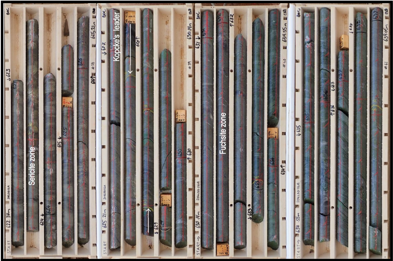
Figure 8: Drill core from hole 20KLDD116A showing Kopcke's leader and the sericite and fuchsite alteration zones.
