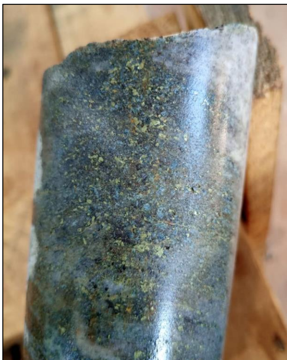
Figure 2 – Detail from CKDD003 exhibiting silicified metagranodiorite highly mineralised with chalcopyrite at 36m
