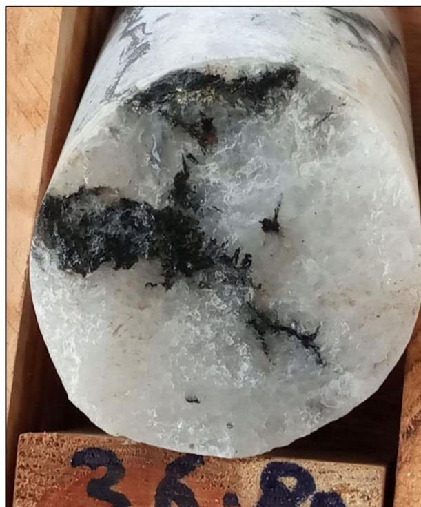
Figure 3 – Detail from CKDD002 at 37m showing tourmaline-pyrite mineralisation within quartz vein zone
