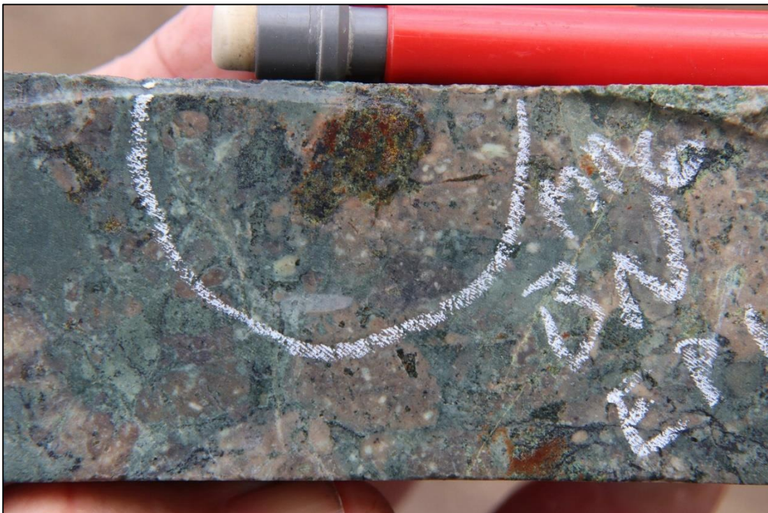
Photo 2. Magnetite-epidote-bornite mineralised clast in the Alfa breccia with potassic altered clasts of dacite porphyry with magnetite-chalcopyrite mineralisation – SMD031, 76.9m.
