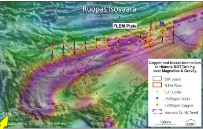
Ruopas Isovaara target comprises a Fixed Loop EM conductor with coincident nickel & copper anomalism in base of till drillholes
