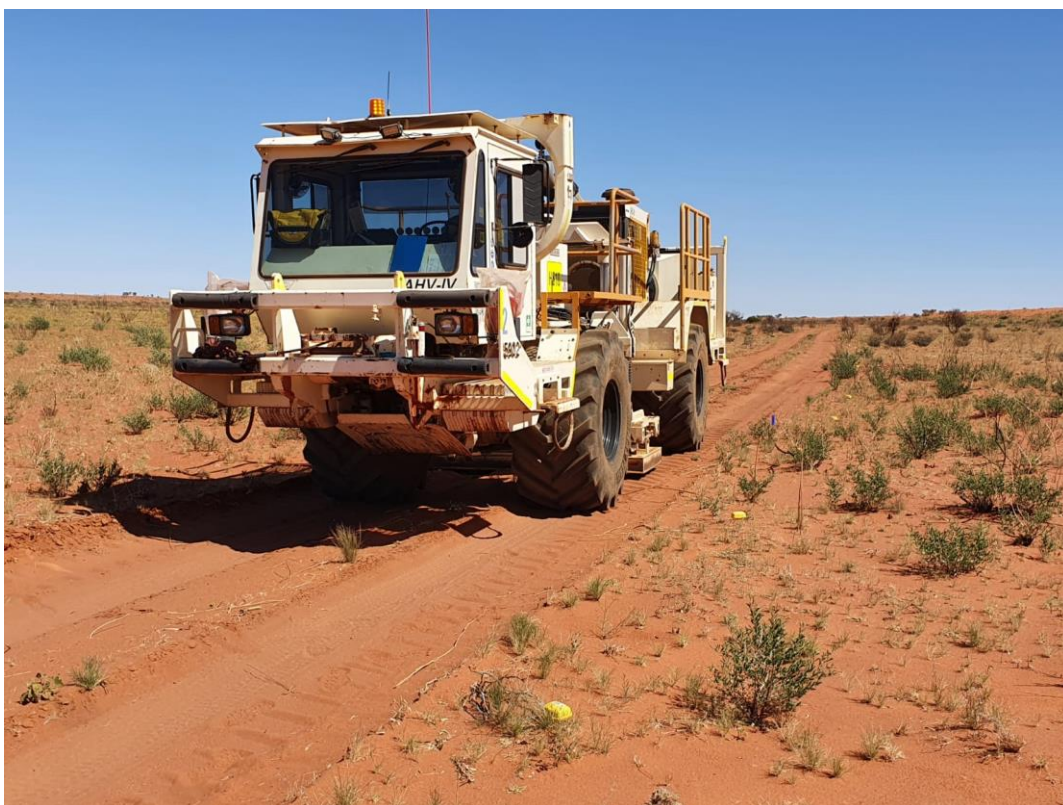
Figure 10 Hiseis Inova AHV-1V 62,000lb seismic vibrator truck with Inova Quantum receiver nodes layed every 5m along the track
