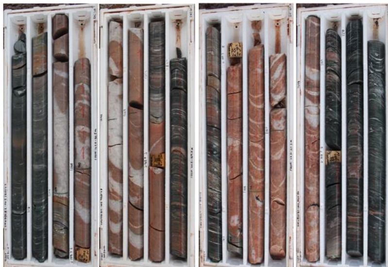
Photo 1: DDH21-1 159m – 168m. 3m @ 11.54g/t Au, within 9m @ 4.49g/t Au, from 159m Mineralisation hosted in silicified quartz porphyry unit with extensive alteration and stockwork veining
