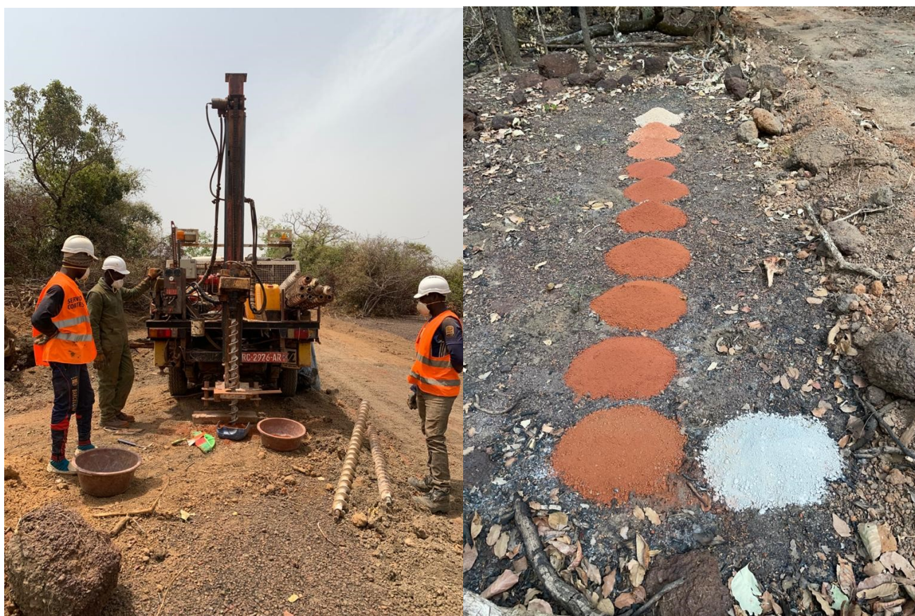
Figure 2. Power auger drilling at Kada. Right hand photo shows 1m samples from a typical hole with laterite cover (red samples) and underlying bedrock samples (cream-grey colour).
