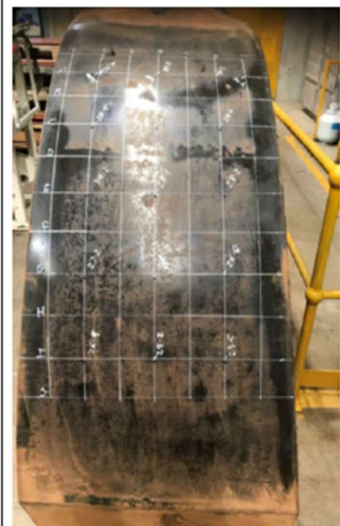
Fig.2c): ArmourGRAPH™ Liner After 62 weeks.
