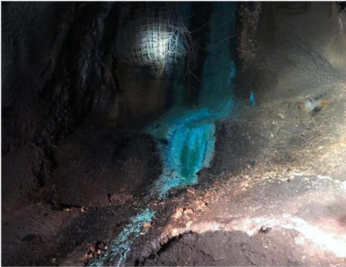
Image 5 / Leached copper in solution from an ore drive at the Nifty underground
