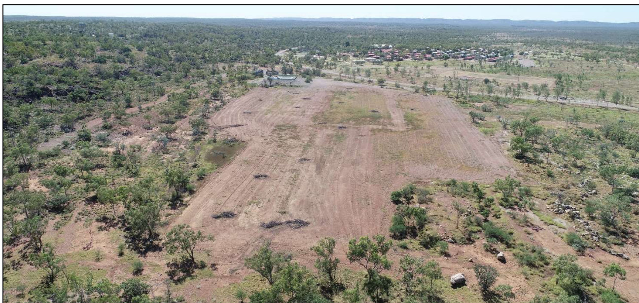
Figure 3: Rehabilitation at the old Century sewerage treatment ponds, with exposed sections undergoing scraping and reseeded to allow regrowth of natural vegetation.
