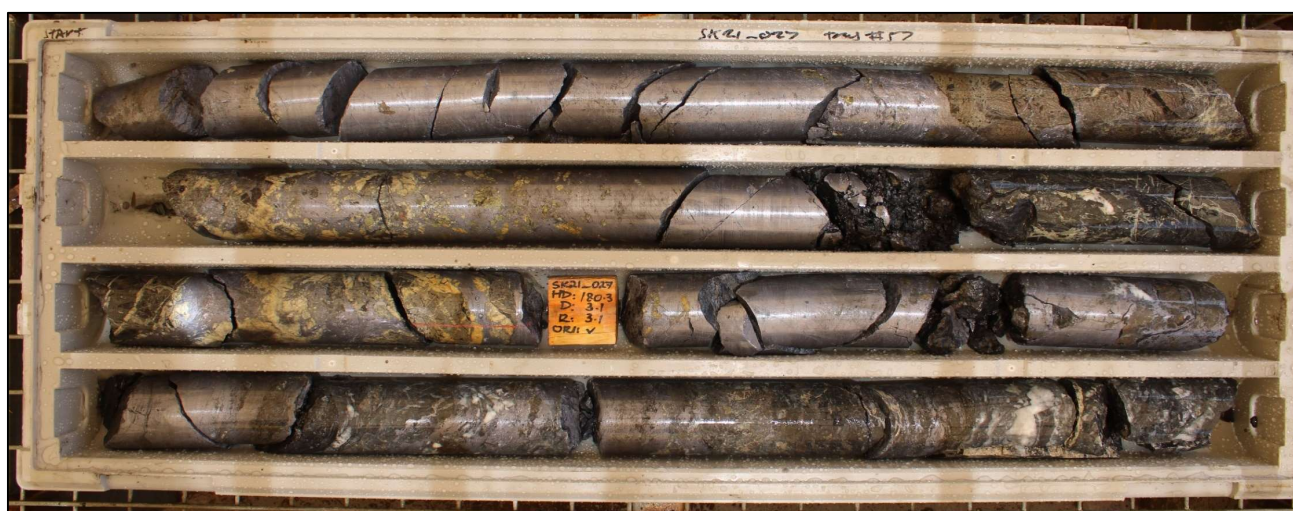
Figure 9: Drill core from hole SK21_027 massive galena showing part of the intersection of 9.5m @ 45.5% Pb, 4.1% Zn, 425g/t Ag from 174.4m
