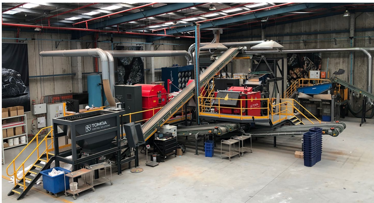
Figure 2. Tomra full size test plant facility in Sydney where 2t drill core and 5t waste dump material was tested. Processing involved on site jaw crusher, screening plant, feed bin, and regulated conveyor system delivering screened material into the Tomra Ore Sorter
