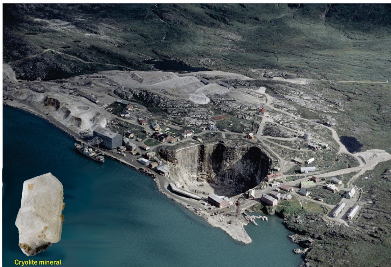
Figure 2: Aerial image of Ivittuut and the cryolite mine in 1960, showing the working open-pit, mine infrastructure, ore and waste dumps and ship loading facilities.
