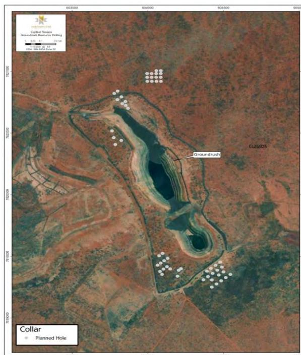
Figure 1 : Groundrush resource infill drill design
