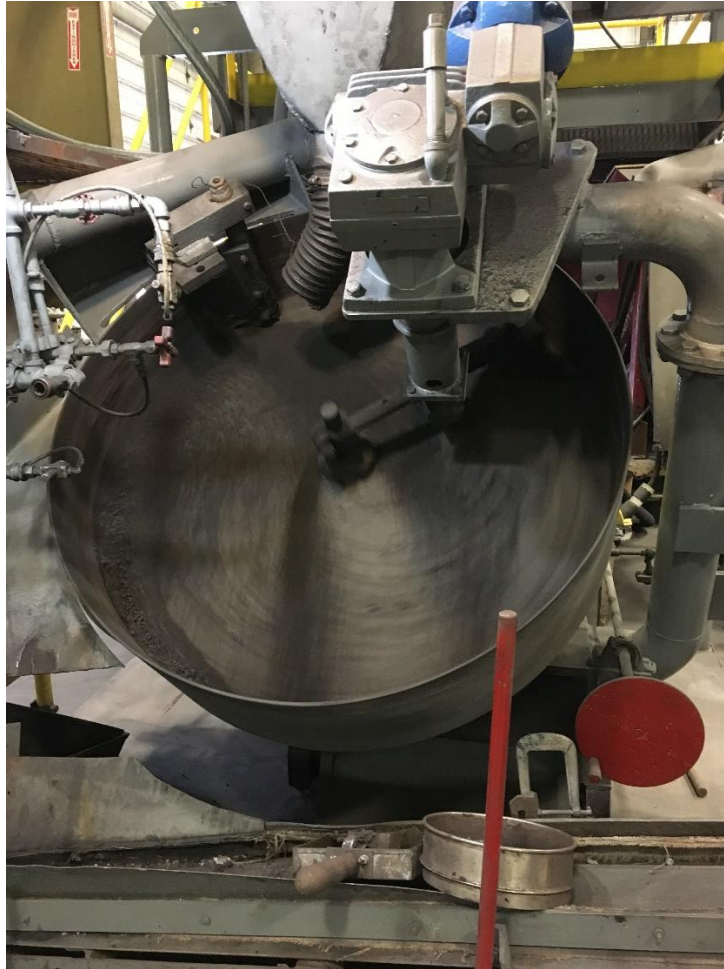
Figure 3 Kiln feed being prepared in pelletising pan
