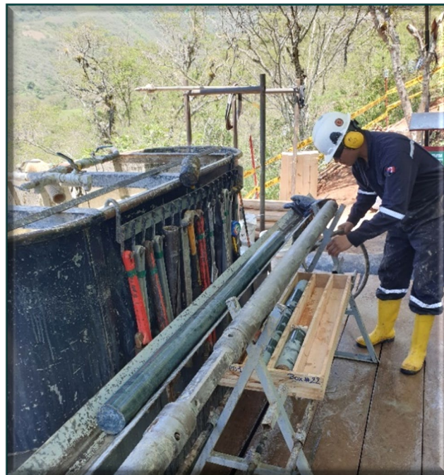
Figure 4: Example of diamond core recovery at drill hole TPD001
