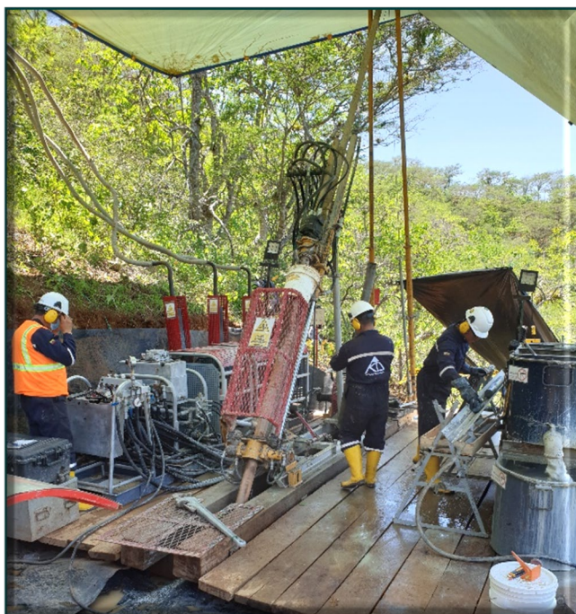
Figure 3: Diamond drill platform at Papayal padsite TPD001
