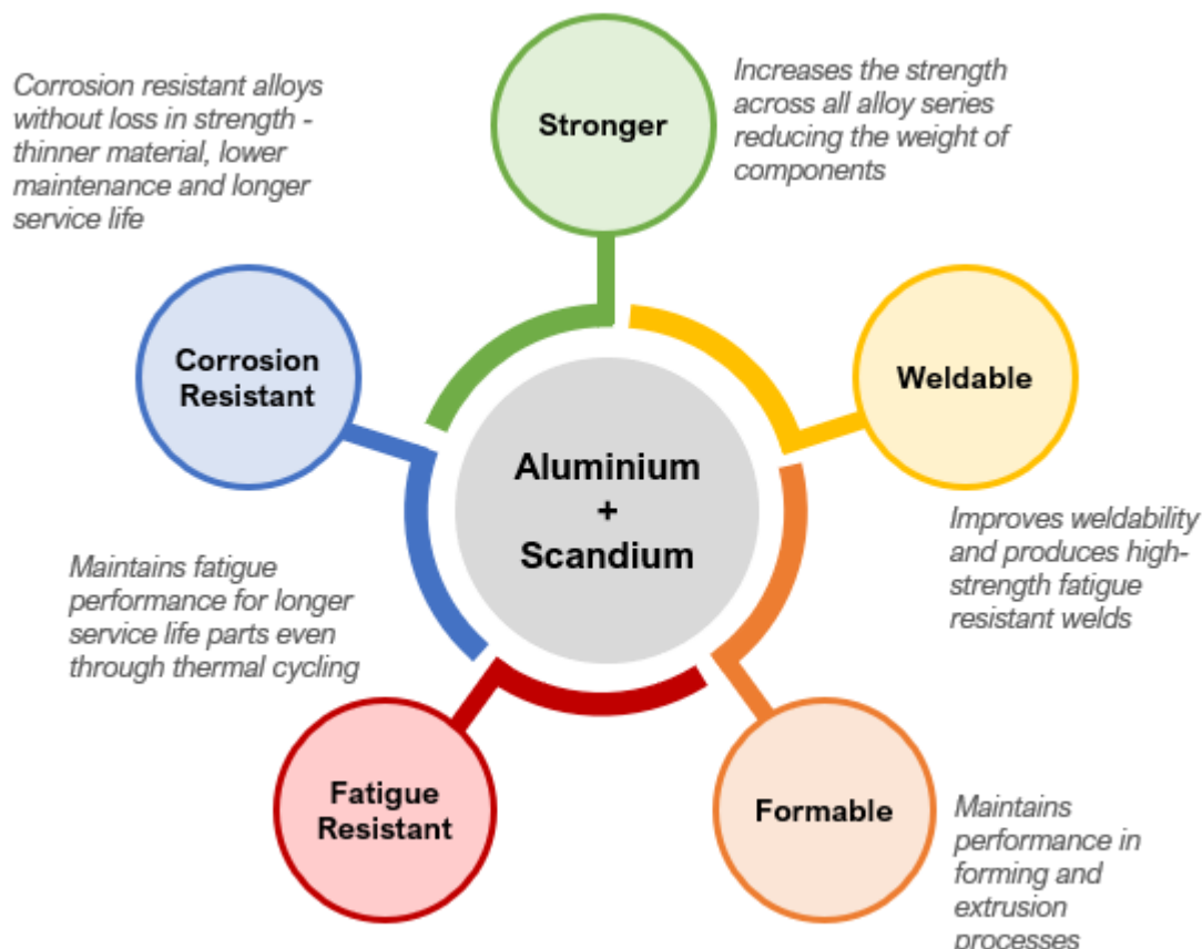
Figure 5: Scandium alloyed with aluminium presents significant improvements to the deployment of aluminium in transportation, enhancing aluminium's leading position in transport.
