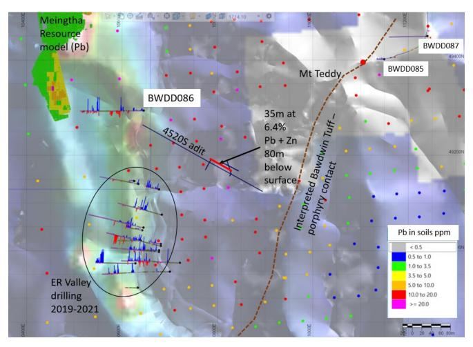
Figure 2 Plan view showing locations of BWDD085-87 at Meingtha South and Mt Teddy. Image of reversed resistivity draped on topography and soil sampling. Of major interest is a possible link between the Meingtha resource and ER Valley drilling highlighted by BWDD086 and a parallel resistivity anomaly. Lead drill hole assay are in blue and copper in red bar graphs.
