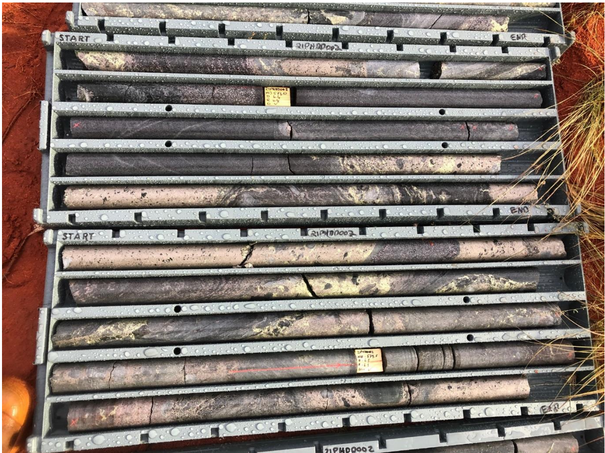
Figure 10: Disseminated, massive and semi-massive sulphide in 21PHDD002 ~570.6-580.7m downhole.
