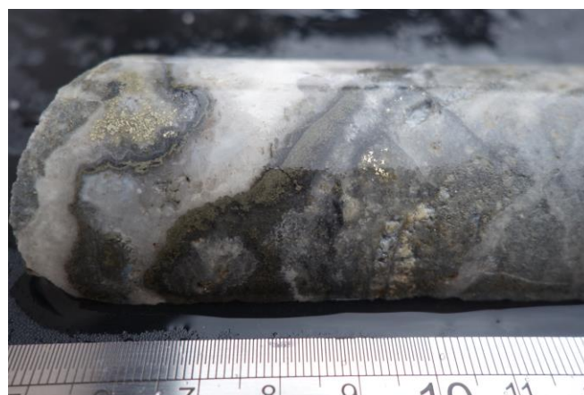
Figure 1: Visible gold in a ~5cm wide, drusy, fine grained, white to grey chalcidonic quartz-pyrite filled vein/stockwork zone at 41.4m in UGA-16
