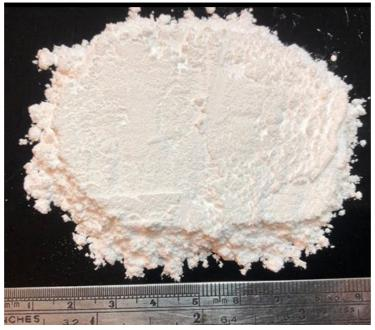
Batch 7 HPA powder product (>99.99% purity) produced from an industrial chemical feedstock
