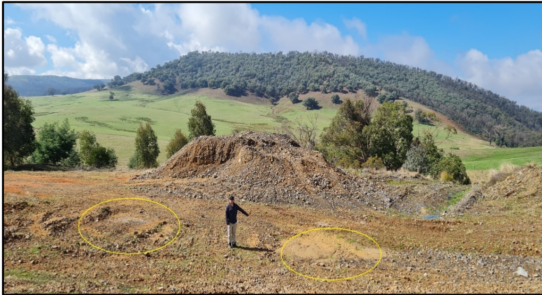
Figure 6: – Partially rehabilitated historic Coppabella Mine (Target Area 4). Yellow ovals indicate the locations of infilled Mine shafts.
