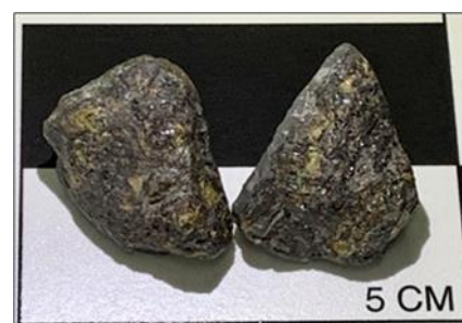
Image 6 – Coarse Grained Massive Sphalerite (Zinc)
