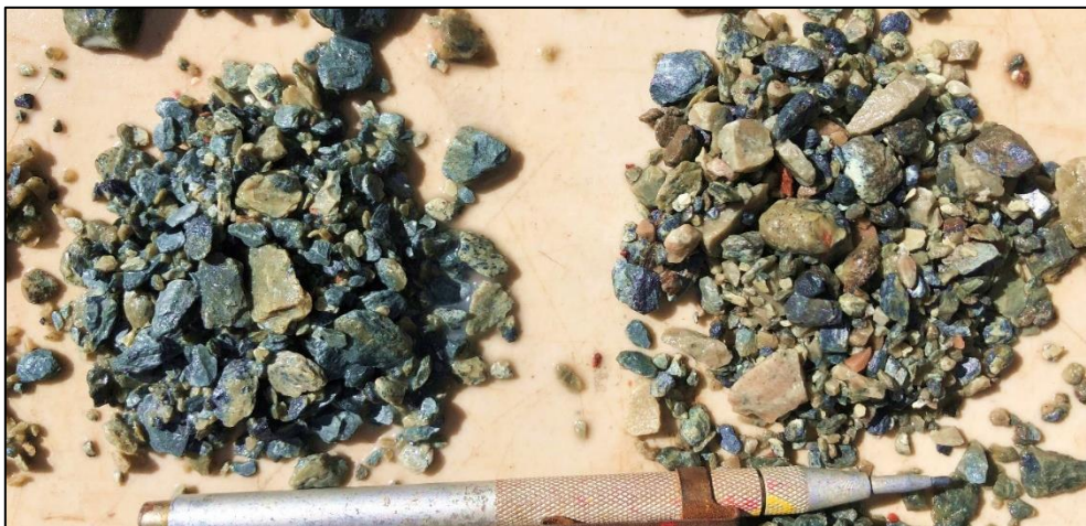
Figure 3: RC chips from hole A3RC004 mineralised interval 89-91m. The grey mineral is galena (lead sulphide), red-brown mineral is sphalerite (zinc sulphide).
