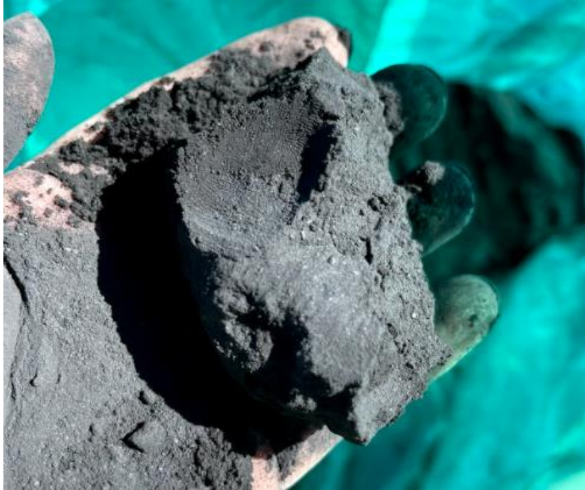
Figure 2. Rich Chalcocite Mineralisation in a Black Powder Unit (supergene zone) from Drill Hole WCRC006 (18-19m) at Powder Hill, Grading 9.5% Cu .
