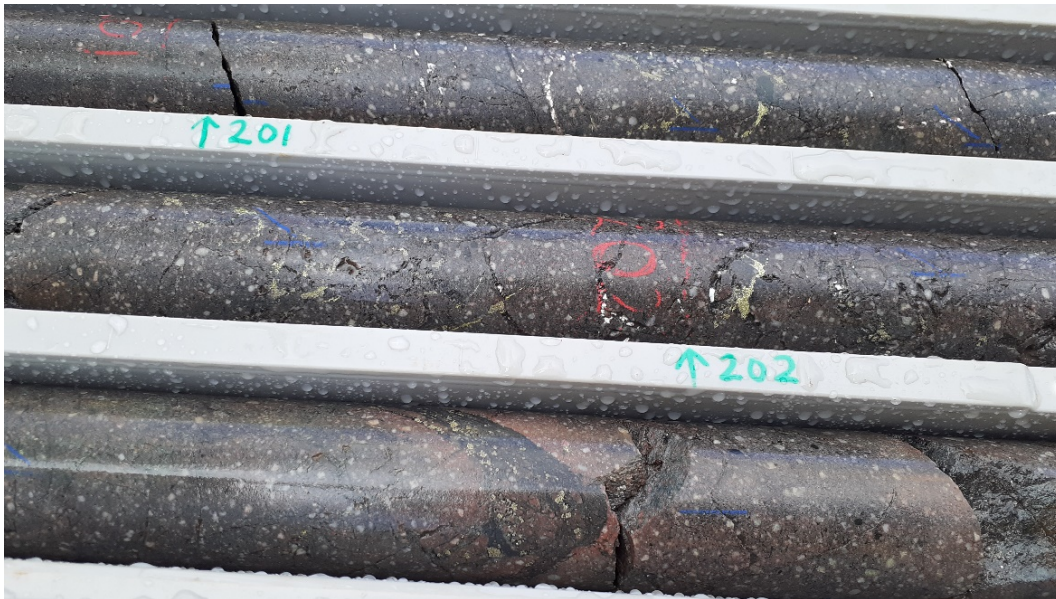
Figure 4 LEFD004 interval 201-203m of altered diorite porphyry with chalcocopyrite and magnetite
