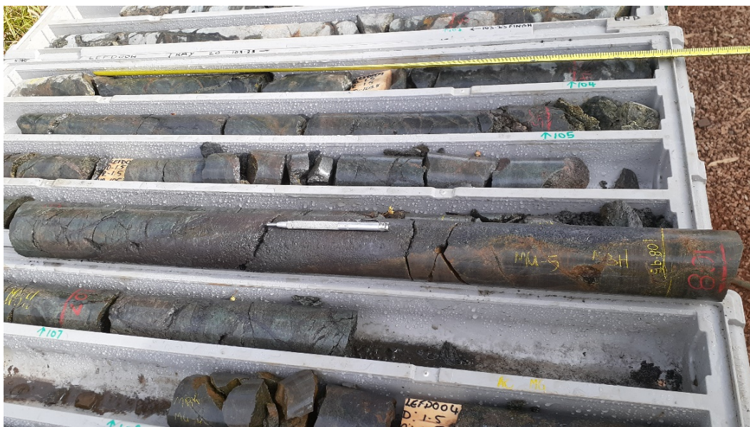
Figure 5 LEFD004 -108m magnetite vein structure (location of pen magnet)
