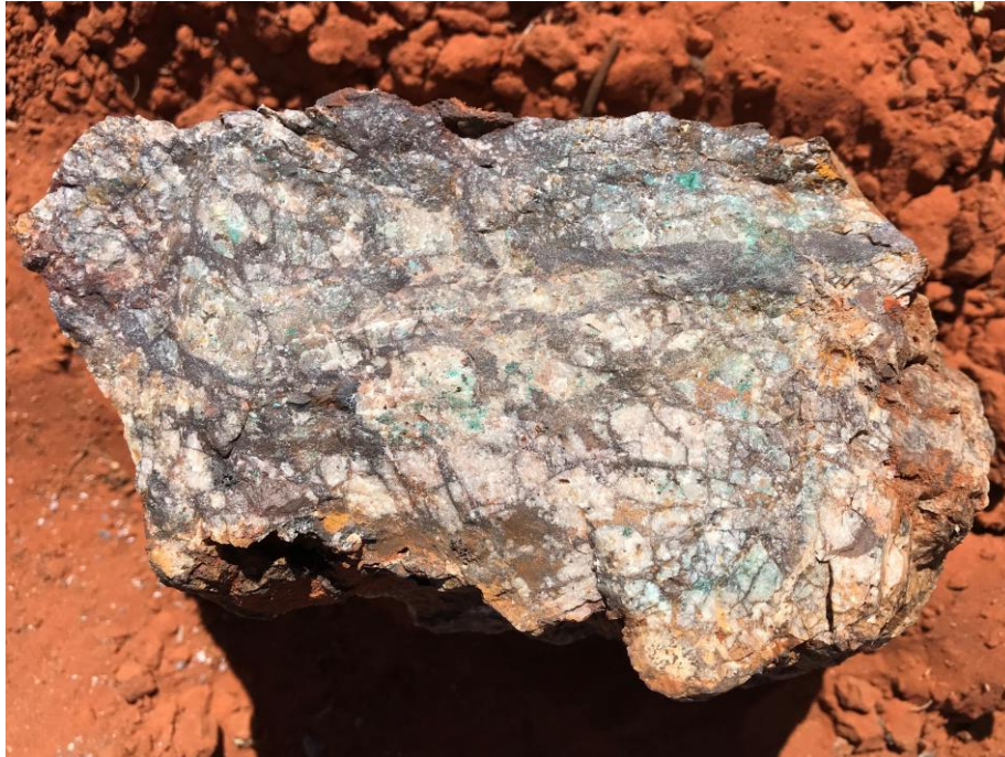
Figure 4. Photo of rock chip sample JE0101 collected at Ningaloo (Figure 3 for location). It is quartz-haematite breccia, the quartz forms the clasts (white) and the haematite from the matrix (red-brown). Disseminated chalcopyrite and malachite occurs in the matrix. This one sample reveals two phases of hydrothermal activity, a first phase of milky white quartz and a second phase of haematite-copper.
