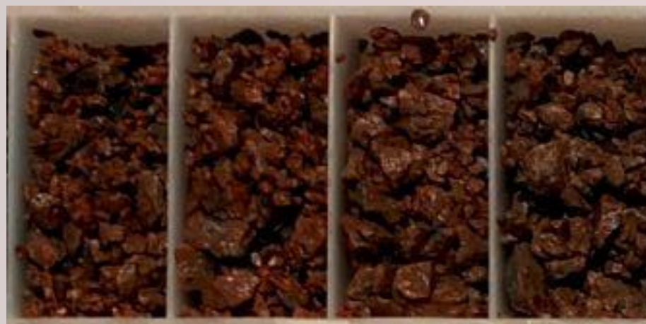
NMWBC18-010 204-208m. 4m @ 2.43g/t Au. Brick-red coloured hematitic alteration at contact of high-level porphyry intrusive and volcanic host rock
