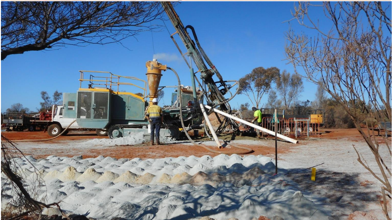
Figure 4: Top – Hydco RC / DD Rig provided by Topdrive Drillers during the coring of CBDD053. Bottom - RC / Diamond Rig provided by DDSR Australia drilling a series of precollars prior to diamond tails.
