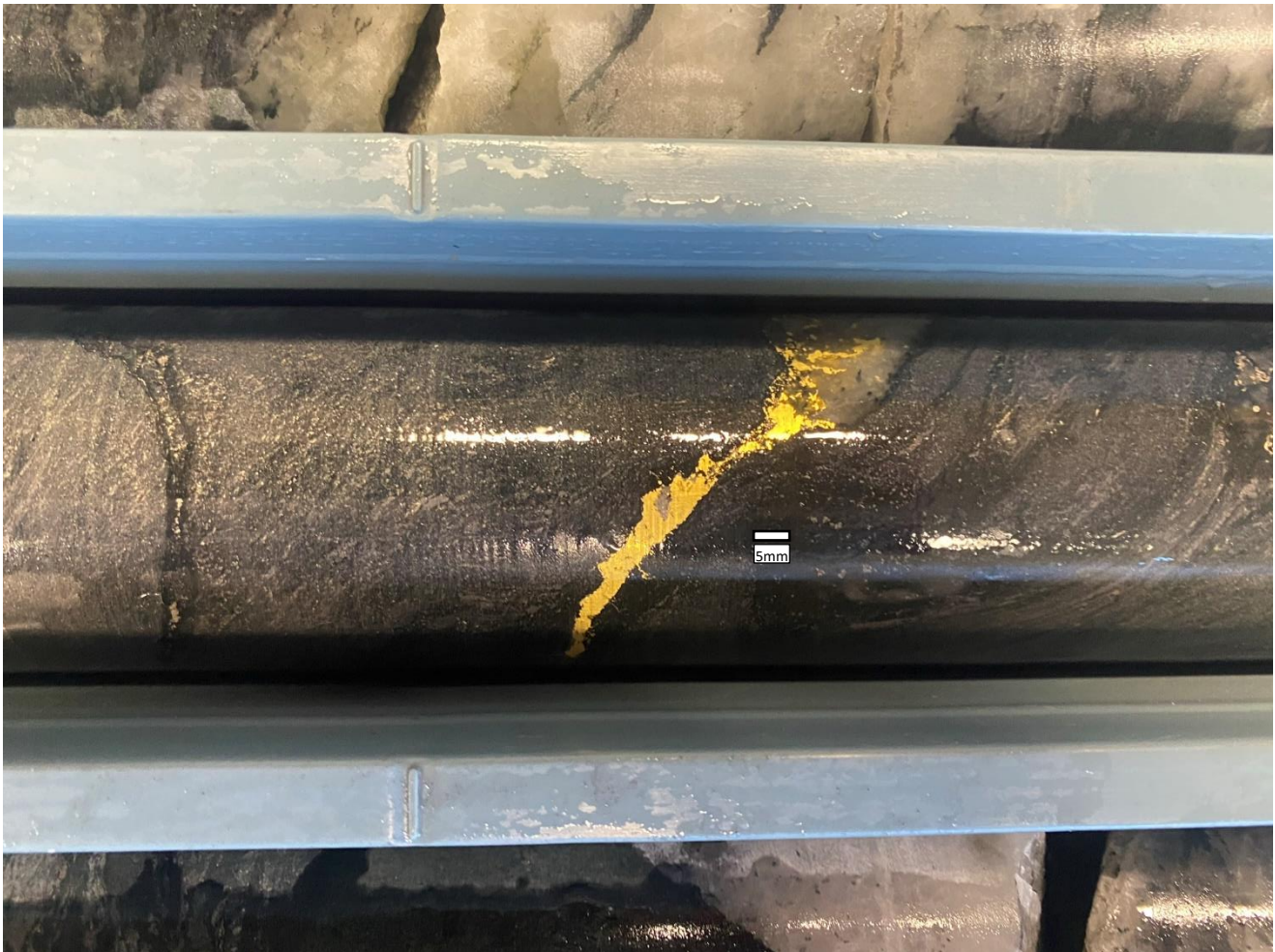
Figure 2. Diamond core from TCKDD0003 with the visible gold at approximately 249m. The gold veinlet is 1mm to 7mm wide and visually appears to be predominantly native gold. Note 5mm scale bar.
