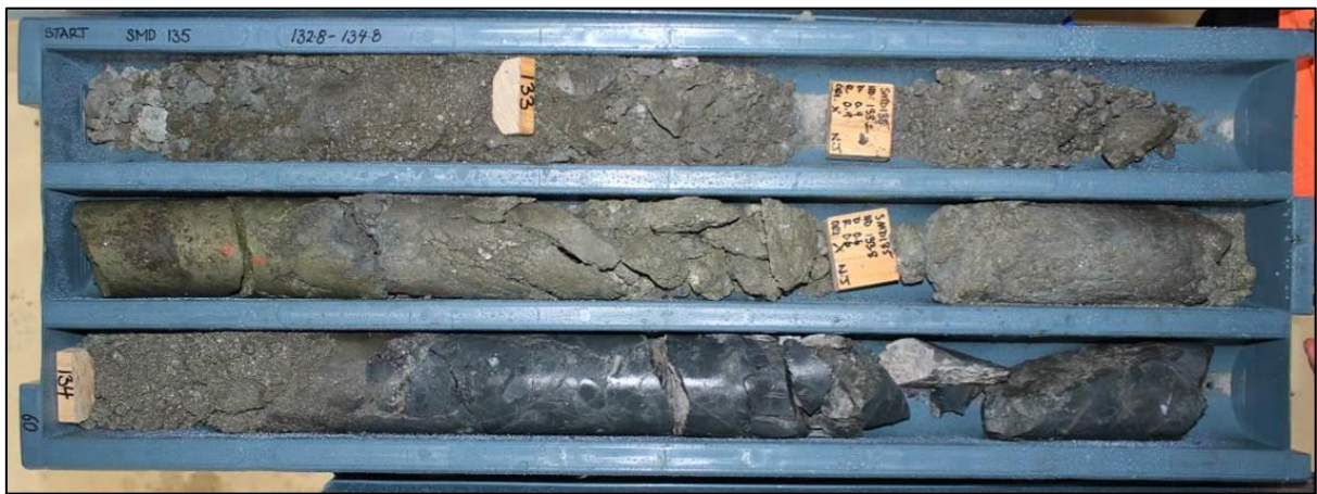
Photo 2. Chalcopyrite and bornite in the Cayley Lode in SMD135.
