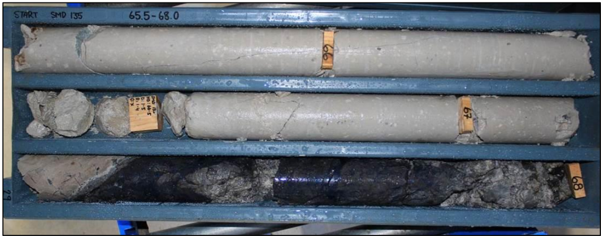
Photo 1. Bornite in the Copper Lode Splay in SMD135.
